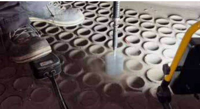
Operator cleaning EGB tubes with AWT-100 and NAB's.
